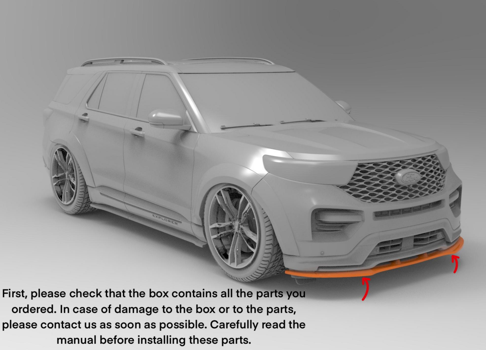
Apply the splitter to the bottom of the bumper and support it with improvised materials so that the splitter is pressed against the bumper.
