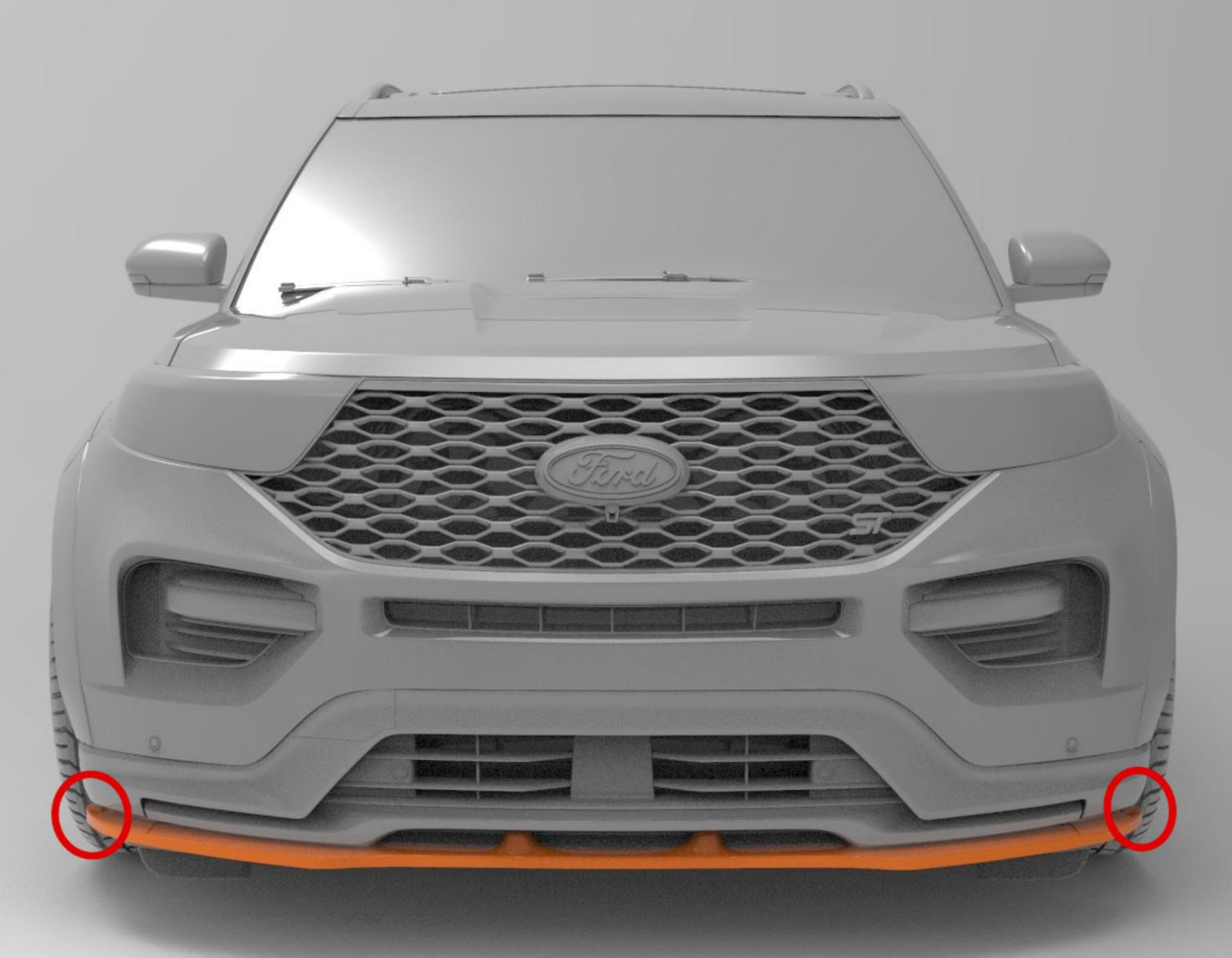
Make sure the splitter is the same on both sides of the bumper.
