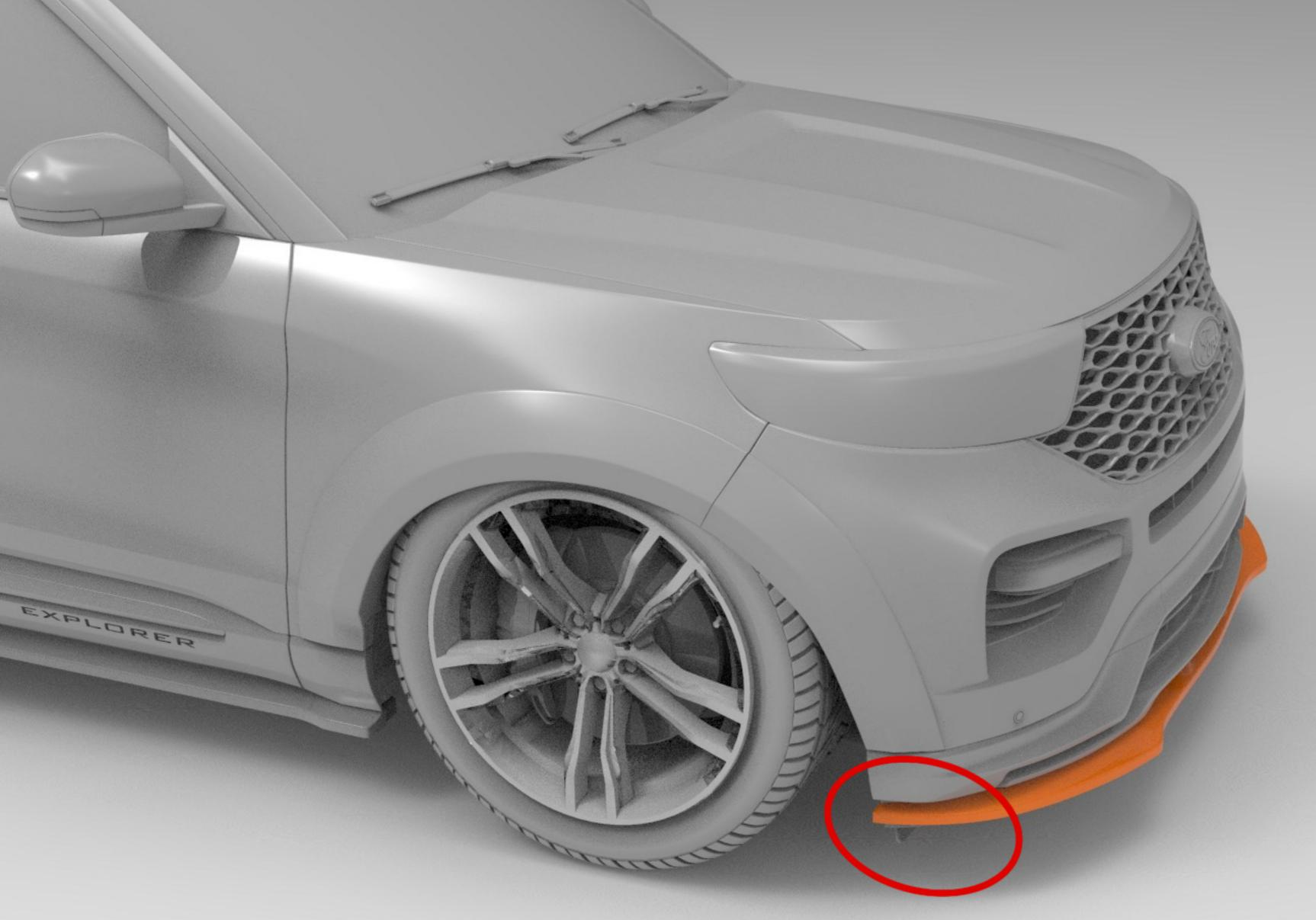
Make sure the splitter is the same on both sides of the bumper.
