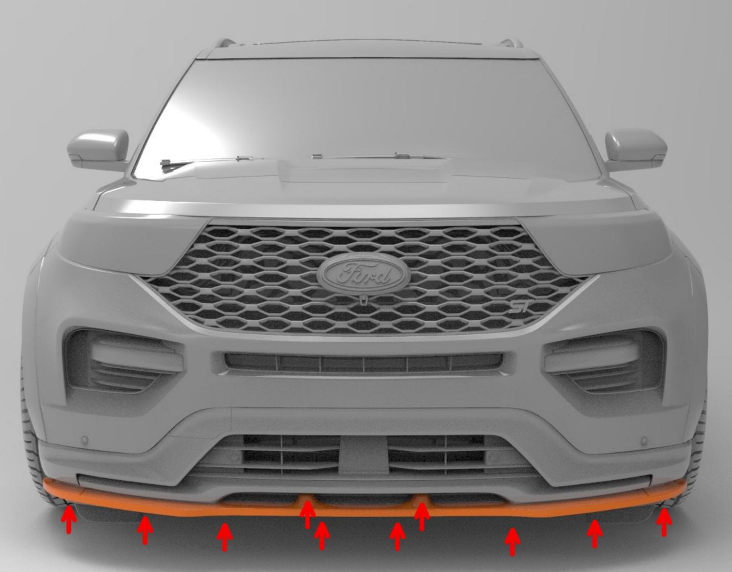
Insert the bolts into all the holes and tighten the nuts on the inside of the bumper. Apply force to tighten the bolts.
