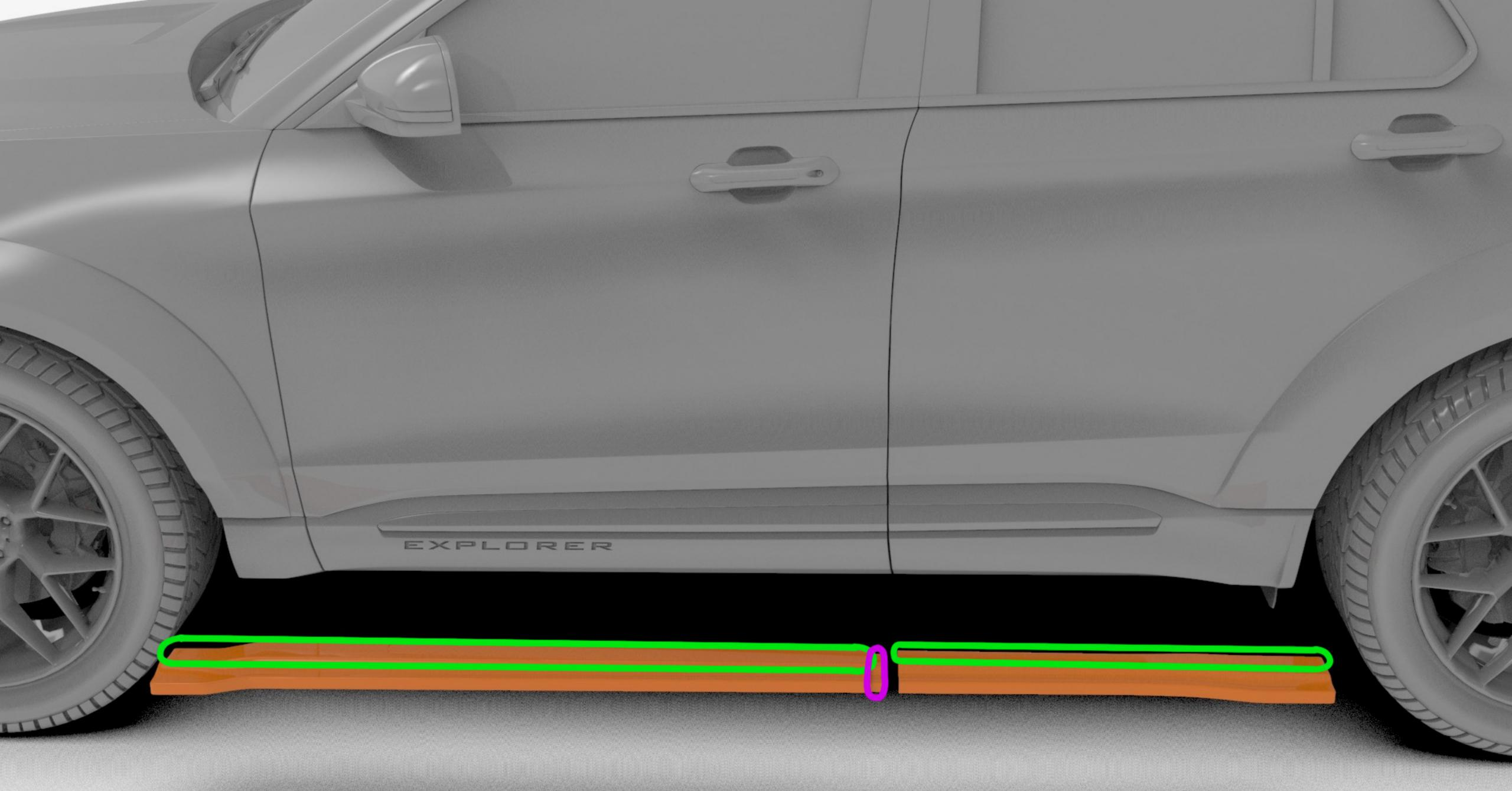
Apply double-sided tape to the area of the side skirt where it touches the original car body (—), apply double-sided tape to the surface of the two parts of the side skirts(—). Double-sided tape should not be too thick, you can use 3m tape. Clean and degrease the original car body at the bottom twice before installation. The surface should be clean and dry.
